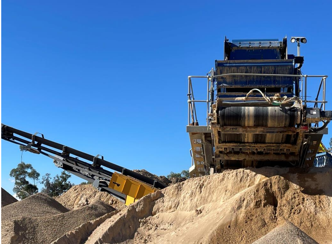
Plate 5 Conveyors on screening plant fitted with water sprays for dust suppression
